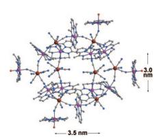
I'll take the high road: An anionic nanosize docosanuclear  $\{Mo_8Mn_{14}\}$  cluster based on the  $[Mo(CN)_7]^{4-}$  unit was synthesized and fully characterized by X-ray and magnetic studies. This molecule (see picture; Mo red, Mn purple, C gray, N blue) is the first discrete compound based on  $[Mo(CN)_7]^{4-}$  and contains the most paramagnetic centers (22) and the largest ground state spin value (S=31) for a cyanide-bridged cluster.
