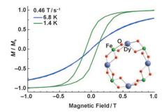
Ferromagnetic interactions in an FeaDya single-molecule magnet were studied using a combination of magnetic susceptibility measurements (see diagram; inset: cluster core) and 57Fe Mössbauer spectroscopy.
